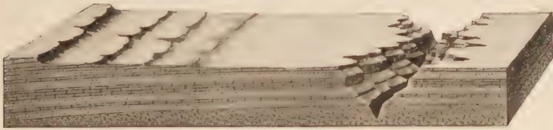
FIG. 73. — A generalized block diagram of the Grand Canyon of the Colorado. The youthful stage of the region is shown in the fact that the streams have as yet accomplished but a small part of the work to be done. The Colorado valley is a young valley. The cliffs of the canyon are formed of resistant beds, while the slopes are of weaker beds.
